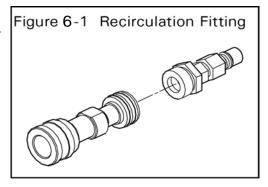
Attach one section of female/female solution hose to the outgoing solution fitting on the front of the machine and the other end to the garden hose and recirculation fitting combination that is attached to the front of the machine(or as many sections as you want, if you wish to freeze guard your hoses).
