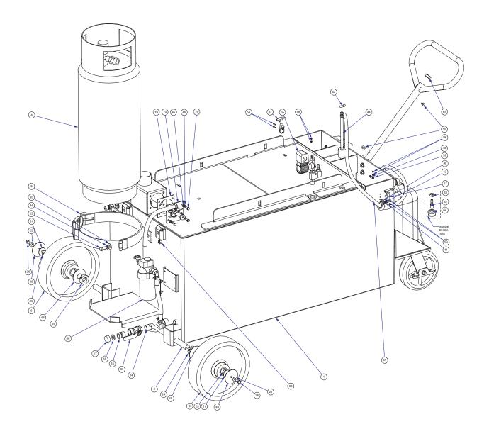
Figure 9-24 Tank Assembly - Front View D-5215 Rev C
