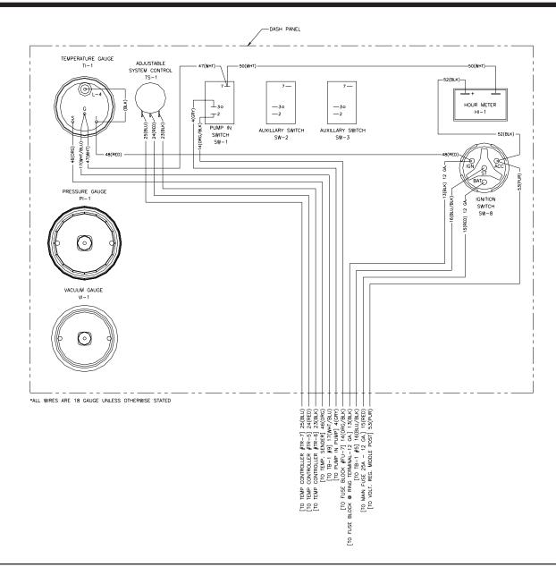
Figure 12-4 **Electrical Diagram**
