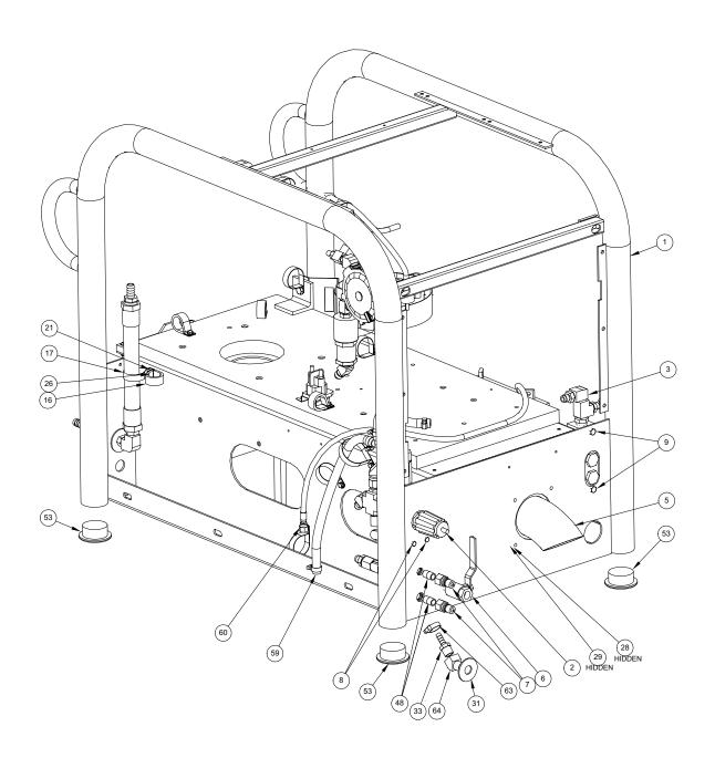
Figure 9-8 Frame Assembly - Rear View - Left Side D-5337 Rev C
