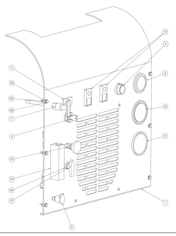
Figure 9-20 Dash Assembly - Rear View D-5339 Rev B
