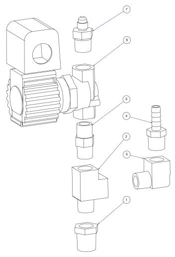
**Dump Solenoid Assembly Parts List**
