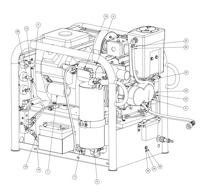
Figure 9-6 Machine Assembly - Bottom View D-5347 Rev A
